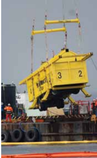
The encased fuel truck at the surface.
